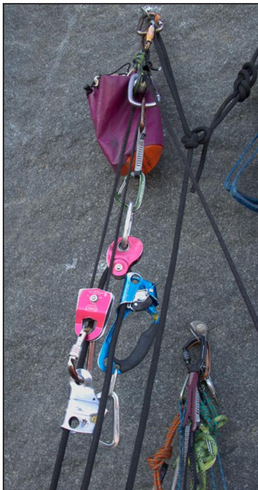
coming from. If there was no Universal, the “Zed Cord”, the cord that runs through your pulleys, would grind on the edge of the top pulley and you would lose efficiency. The Zed Cord can be 5 mil Spectra cord, but be careful, Spectra cord is pretty delicate and can easily abrade and break on one route. There is a new kind out, I don’t know it’s name but it doesn’t stretch and resists abrading far better. You’ll want Spectra because it is strong and doesn’t stretch.
